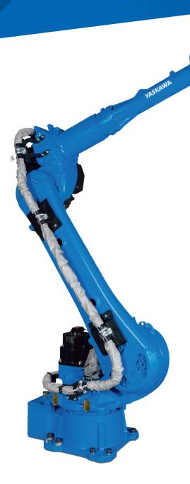
The fast and dynamic 6-axis MOTOMAN GP70L robot offers top performance for order picking as well as item, box and carton handling in the logistics industry. The most powerful robot in its class offers a huge increase in terms of efficiency and productivity for sorting and packing in intralogistics applications.
