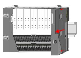
**1.** Before mounting the periphery modules you have to remove the bus cover at the right side of the CPU by pulling it forward. Keep the cover for later mounting.
