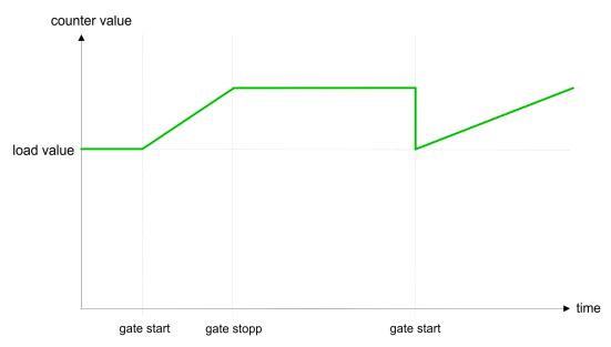
At *interrupt function*, the counter starts counting with the last recent counter value after gate restart.
